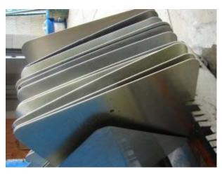
Northwest Sign Recycling inventories the signs, hydrostrips them, deburrs any rough edges, and returns the refurbished sign blanks to the City.
