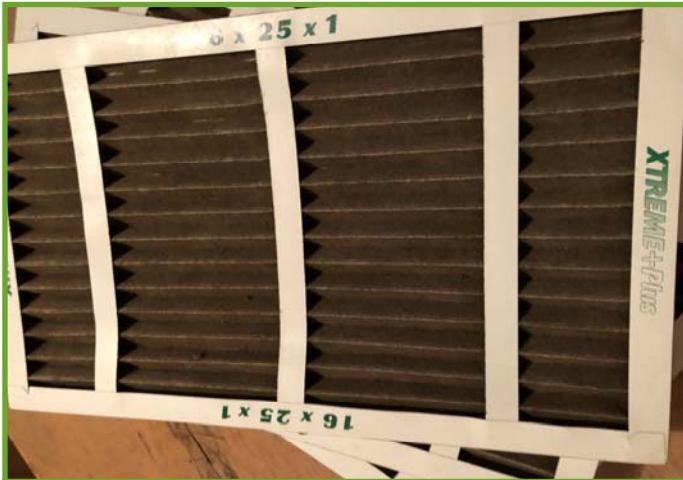
Old filter - discolored by smoke
