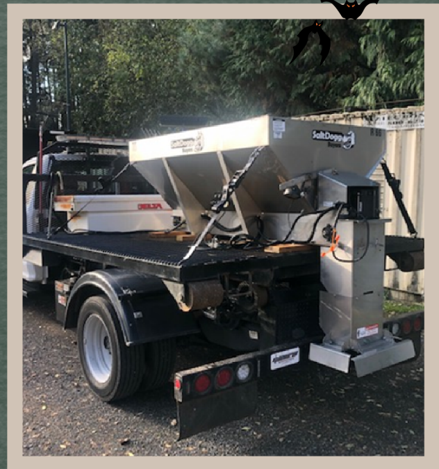
New sand spreading unit, installed and ready for service.
