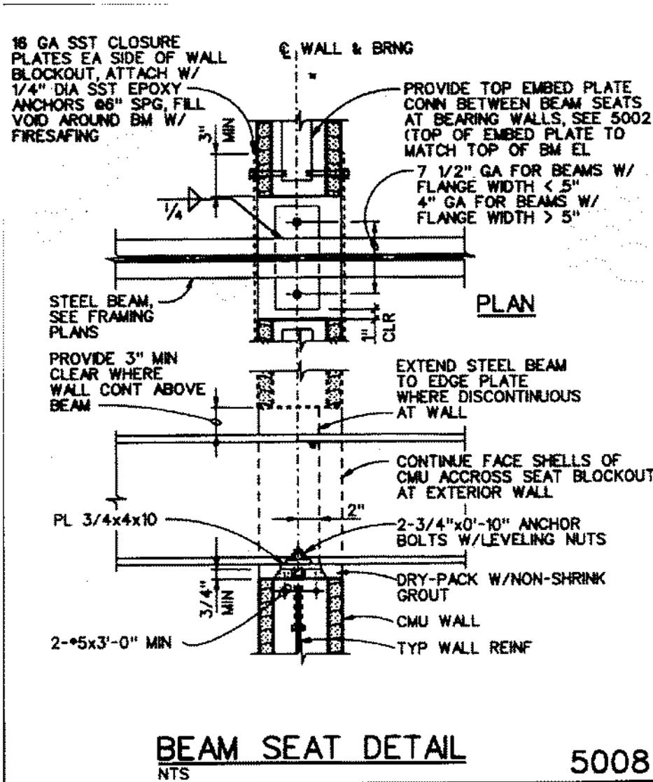
BEAM ANCHORAGE CONNECTION DETAIL ALONG EAST AND WEST WALL ELEVATIONS
