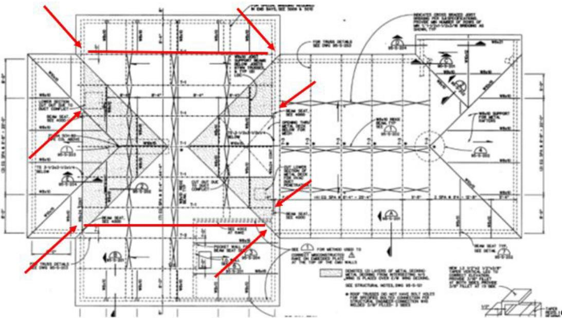
Figure 4 Operations Building - Drag Connection Deficiency Locations
