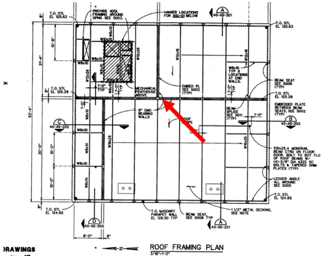
Figure 1.3 Process Gallery - Collector Beam Location and Anchorage Deficiency
