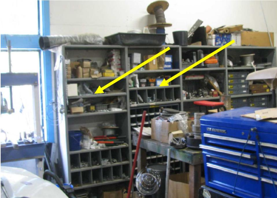
Figure 23 Workshop - Storage Shelves on South Wall Missing Anchorage
