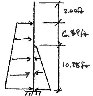
For soil pressure on wall, assume a load of 40pcf triangular. See attached spreadsheet for hydrostatic & hydrodynamic loads on wall.
