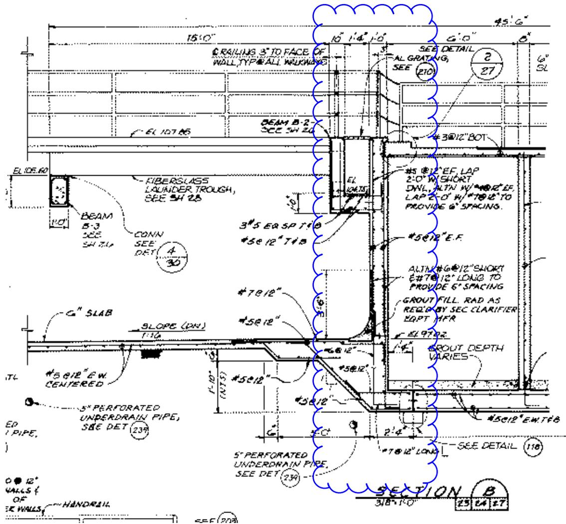
Dividing Wall between Biofilter and WAS Basins
