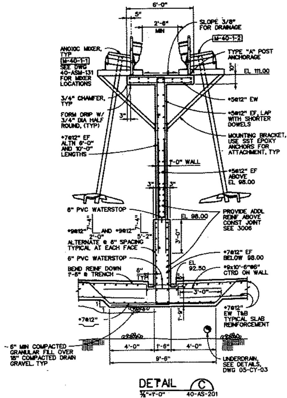
Dividing Wall Section Reinforcing
