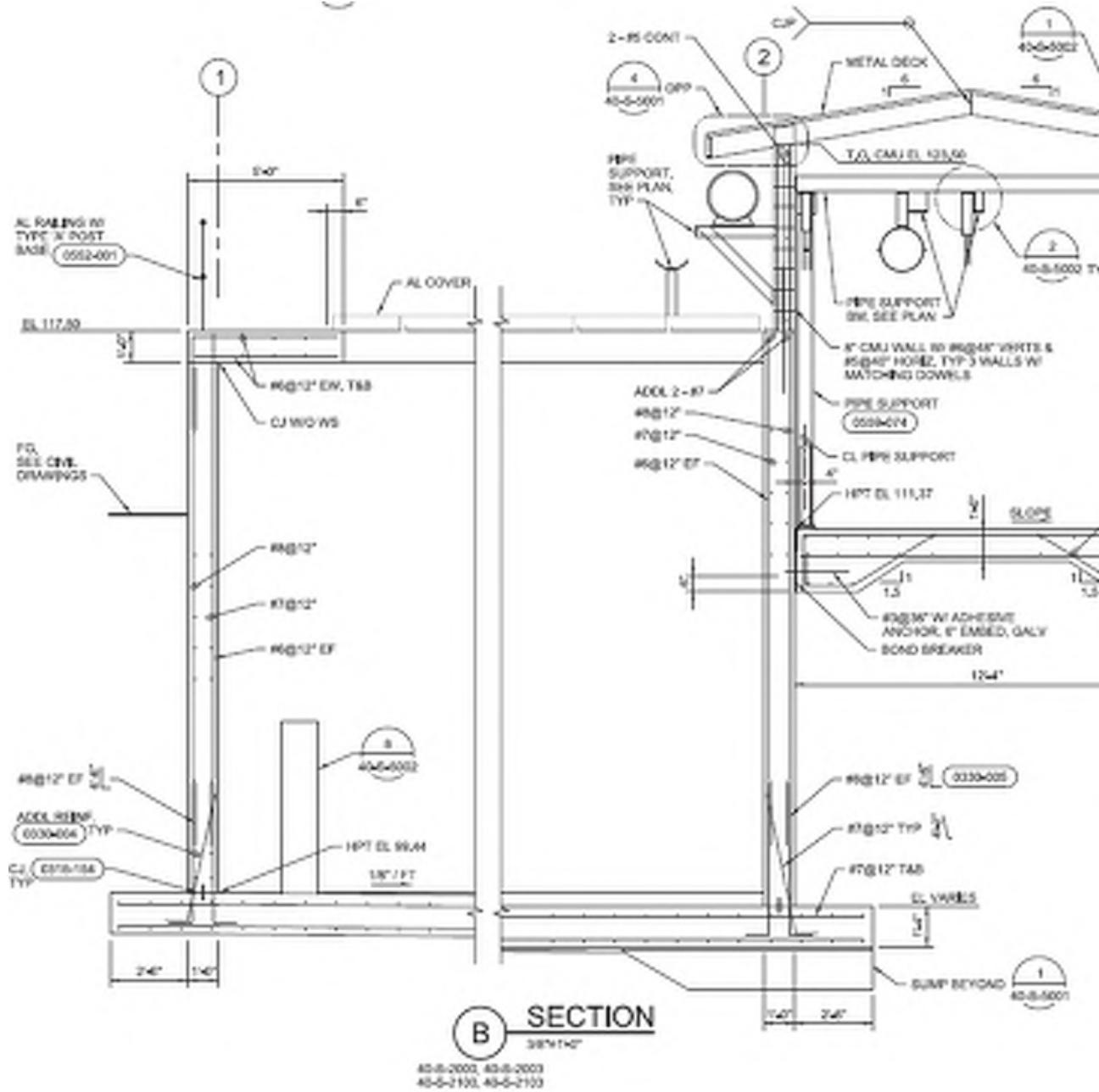
Stabilization Basin Perimeter Wall Section Reinforcing
