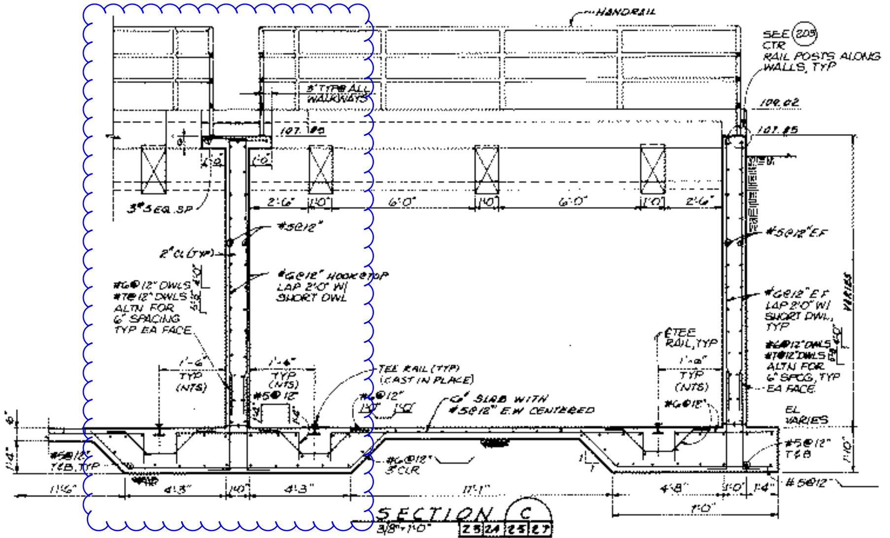
Dividing Wall Section Reinforcing
