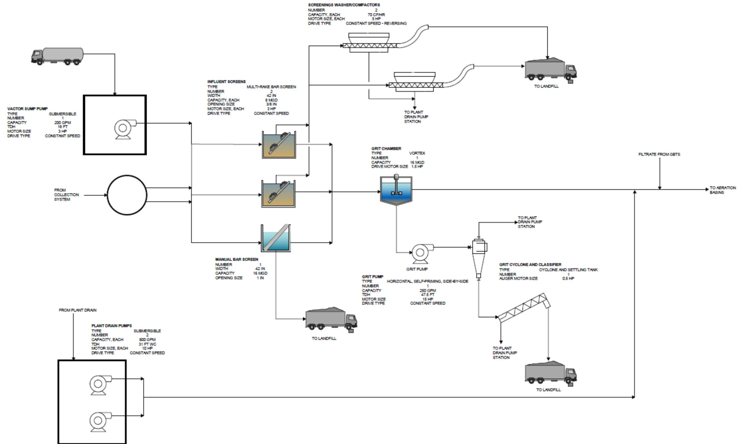
Figure G.1 Preliminary Treatment Schematic
