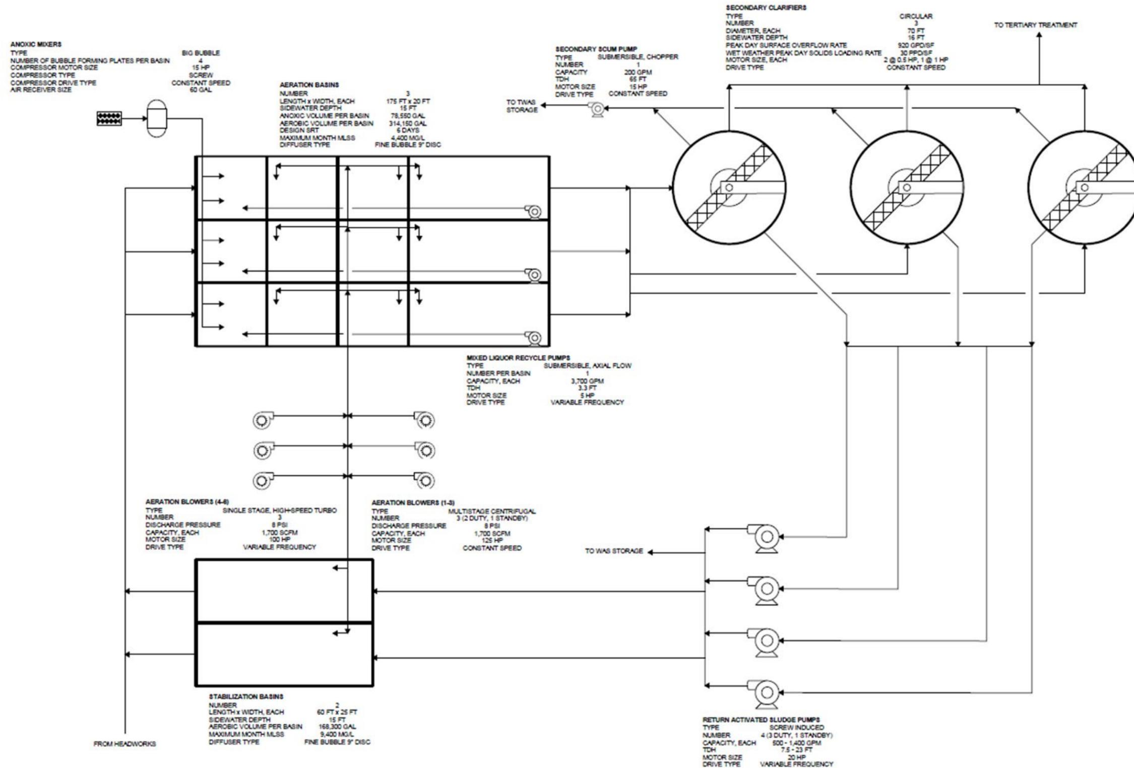
Figure G.2 Secondary Treatment Schematic
