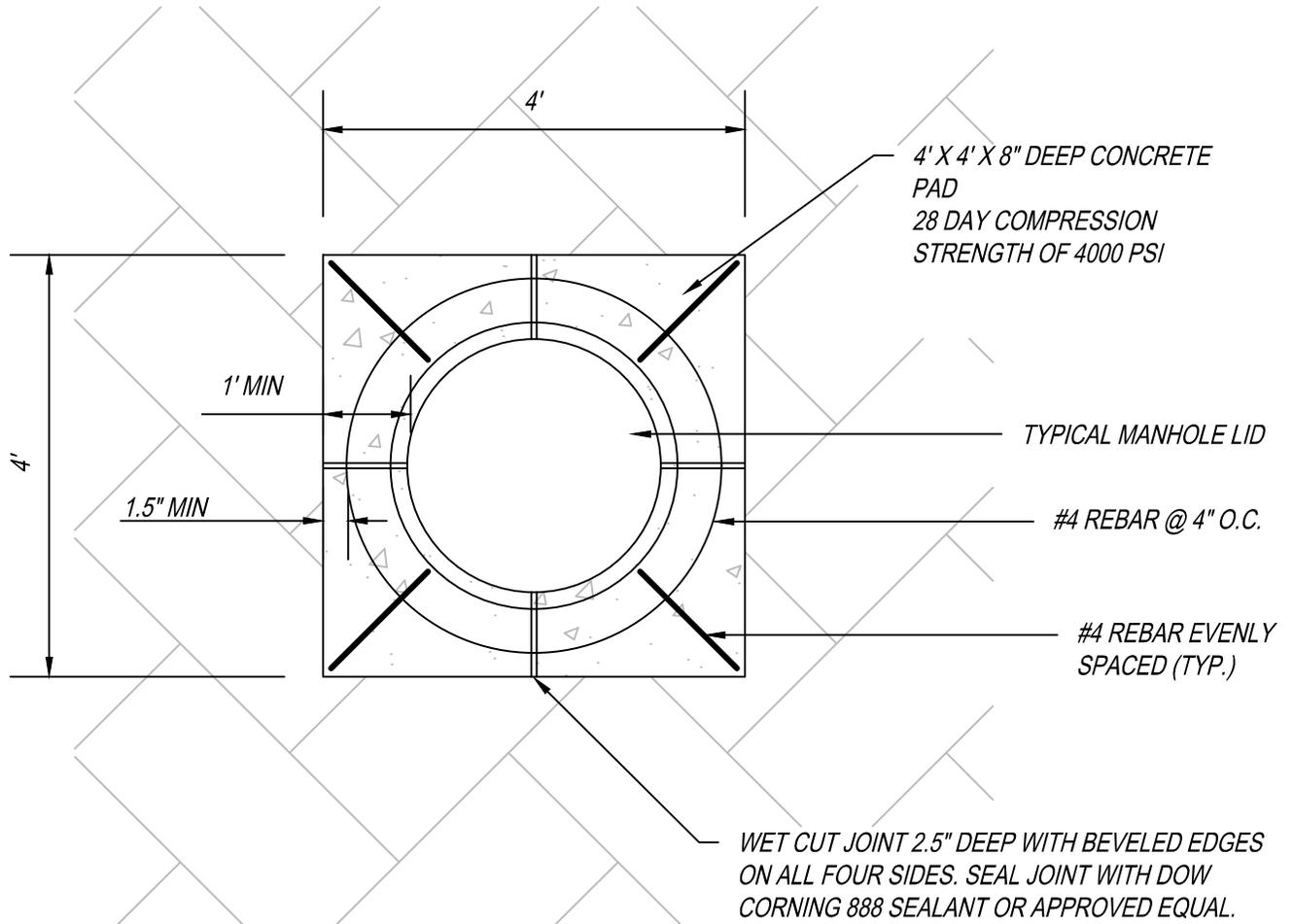
Manhole Collar For Pervious Pavement
