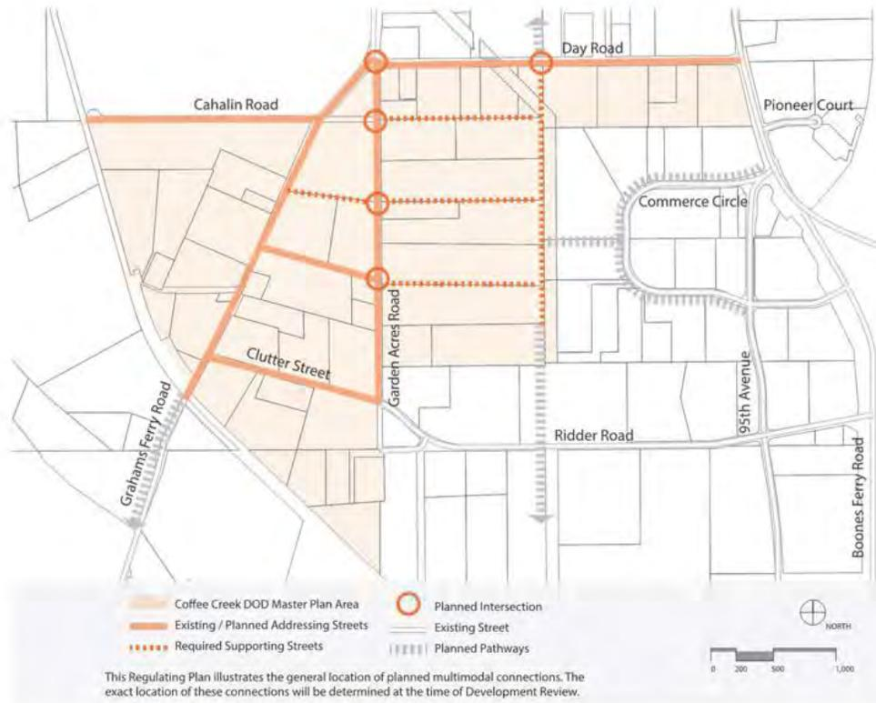
Figure CC-1 - Regulating Plan
