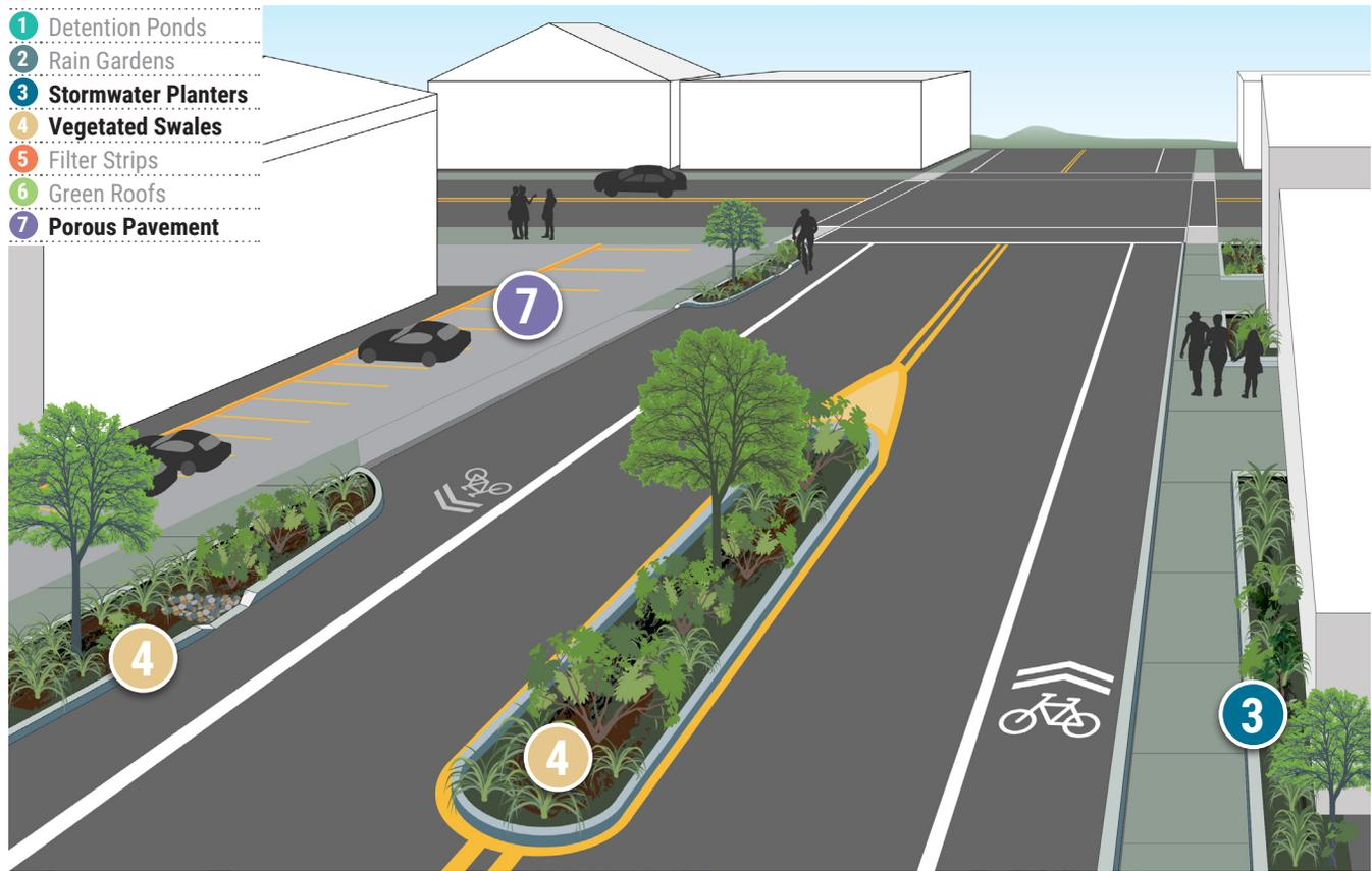
Example of stormwater management facilities applied to a transportation corridor. Applicable facilities are highlighted, as not all types of facilities may be used at a site.
