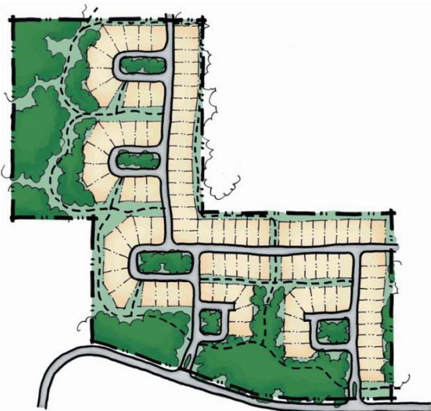
Clustered housing, narrow lot frontages, and looped roadway design can reduce impervious areas and increase open spaces in proposed site layouts.
