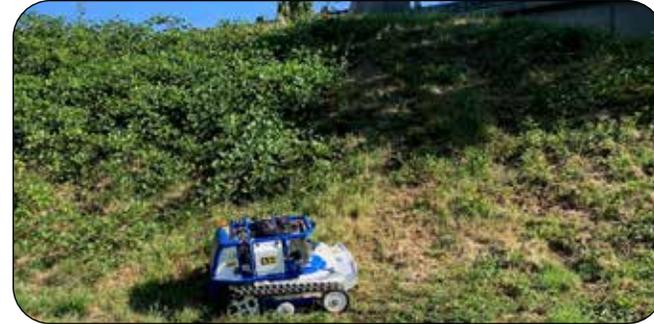
With a remote slope mower, City Road Maintenance crews can safely mow blackberry on dangerous inclines or other hard-to-reach places.
