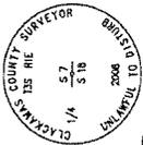
FOUND 3-1/4" BRONZE DISK DOWN IN A WOODPILE BOX (U.S.G.T. 2008-09) AT THE NORTHWEST CORNER OF SECTION 18, FIELD STAMPED AS SHOWN.
