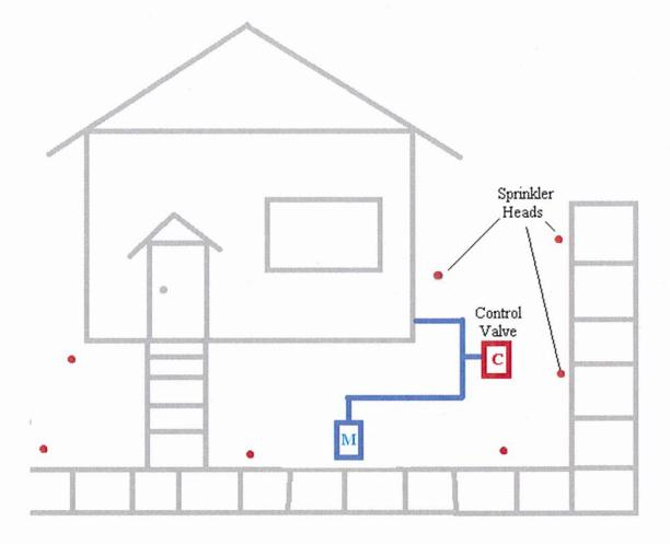
If your water usage is high but there is no movement on your meter you may have an irrigation leak. When the pipe breaks between the meter and the house the meter will constantly register water flow. Toilet leaks may show as intermittent leaking on the meter. If the mechanism in the back of the toilet doesn't seal properly it can allow water to seep into the bowl constantly. When the reservoir tank gets low enough it will refill. A common misconception is you will hear the problem.
